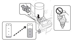
**Note:** If ink does not flow from the bottle, lift and reinsert the bottle.
