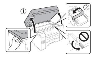
**Caution:** The printer ships with the transportation lock in the printing position. Do not move it from the printing position.
