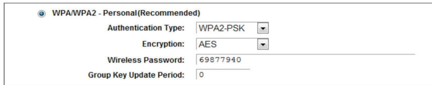
The screenshot shows the configuration interface for WPA/WPA2 - Personal. It includes a radio button for selection, and several fields: Authentication Type (WPA2-PSK), Encryption (AES), Wireless Password (69877940), and Group Key Update Period (0).
