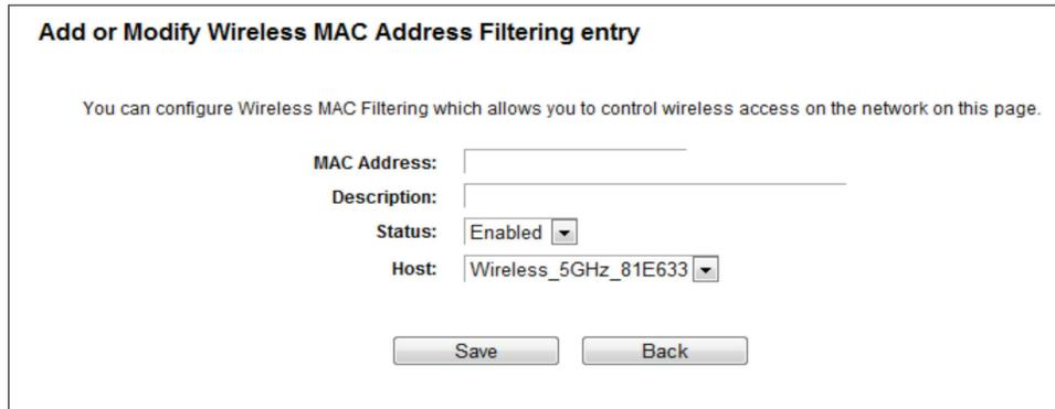
The screenshot shows a web form titled "Add or Modify Wireless MAC Address Filtering entry". Below the title is a sub-header: "You can configure Wireless MAC Filtering which allows you to control wireless access on the network on this page." The form contains the following fields and controls:
