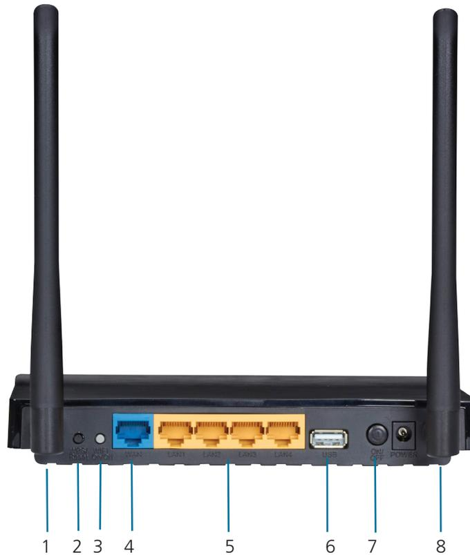
Figure 2-2. Router's back panel.
