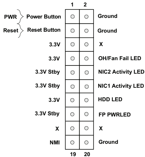
Figure 3-1. JF1: Control Panel Pins
