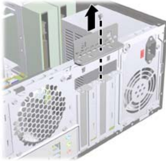
Figure 7-7 Opening the Slot Cover Lock
