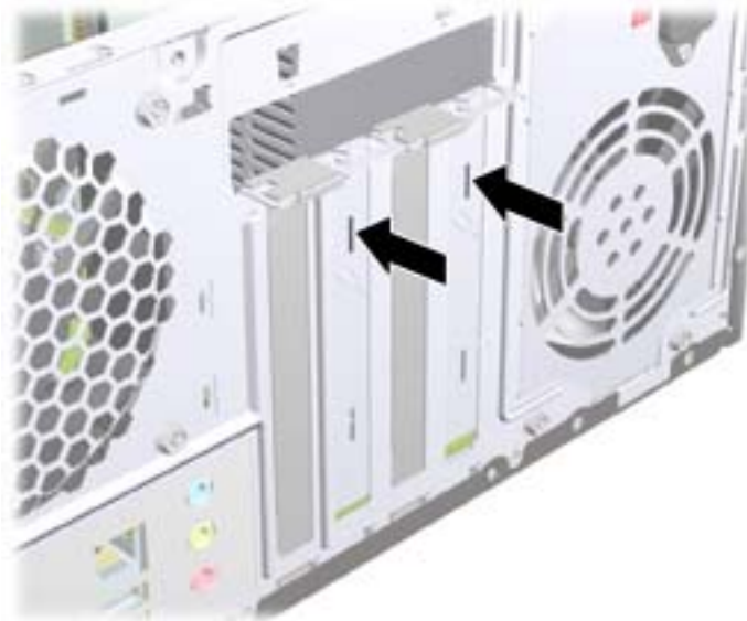
Figure 7-8 Removing an Expansion Slot Cover
