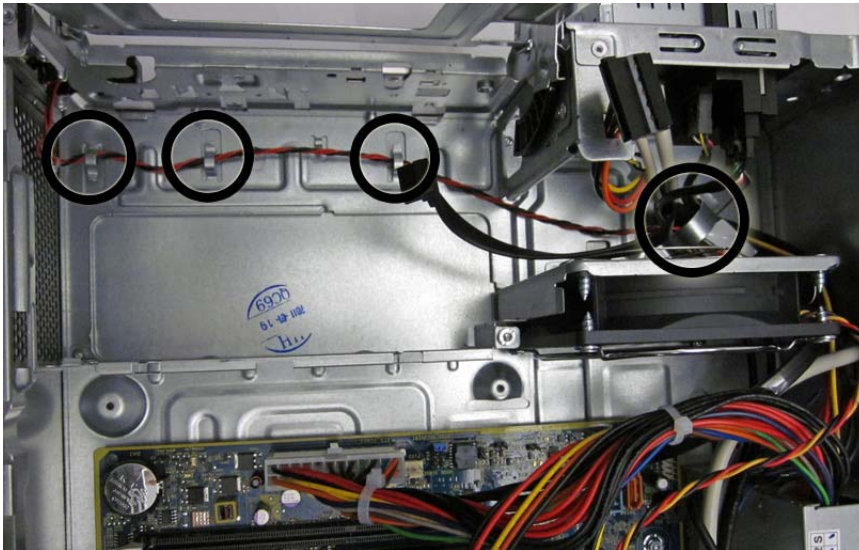
Figure 8-23 Removing the power switch cable
