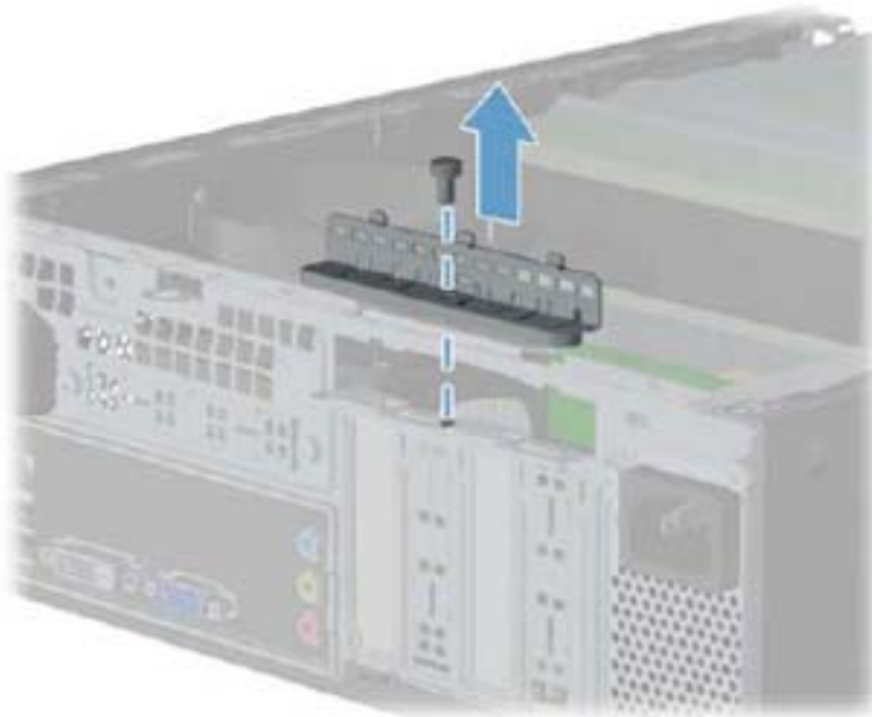
Figure 8-10 Opening the expansion slot bracket
