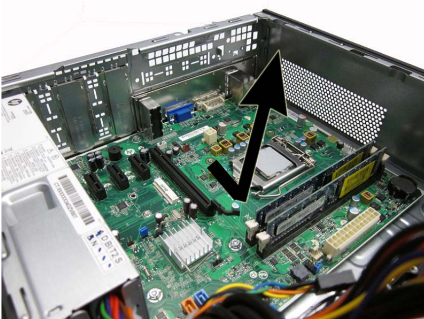
Figure 8-38 Removing the system board
