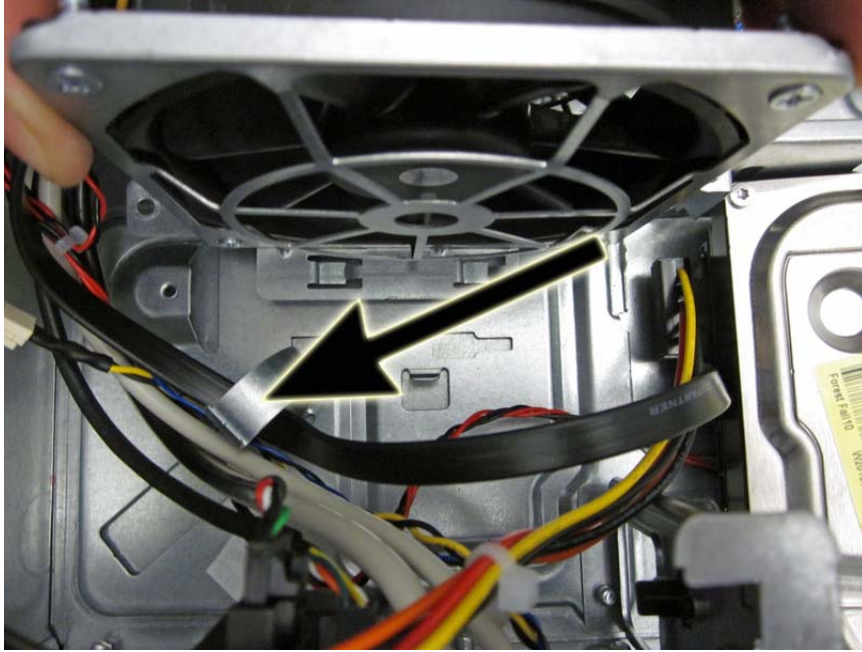
Figure 8-27 Removing the cables from the clip
