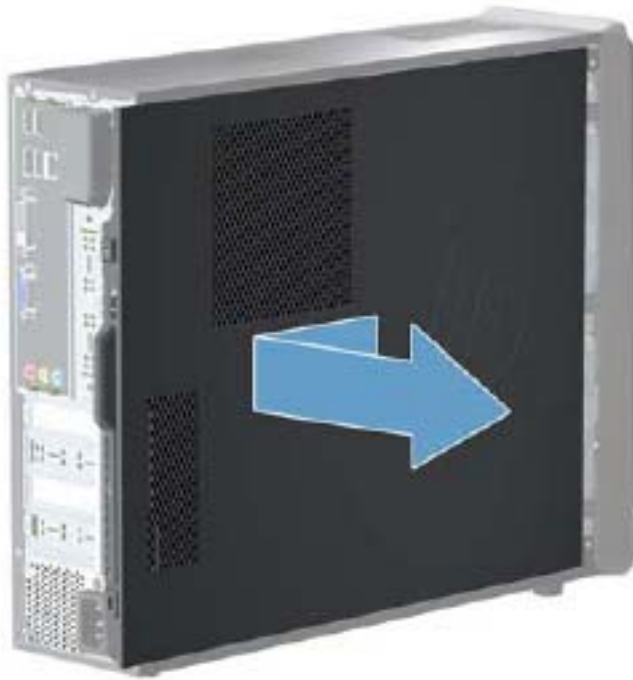
Figure 8-2 Removing the access panel
