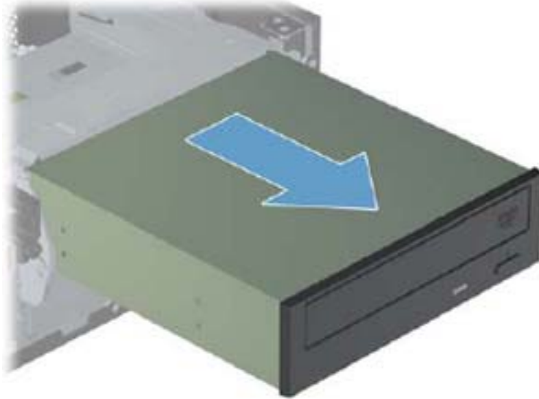
Figure 8-17 Removing the optical drive
