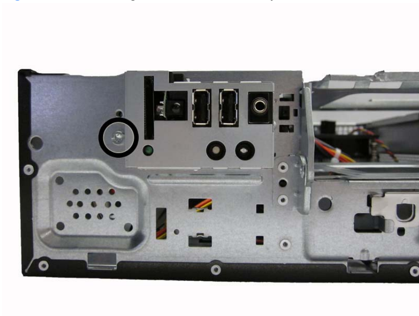
Figure 8-28 Removing the front USB assembly screw
