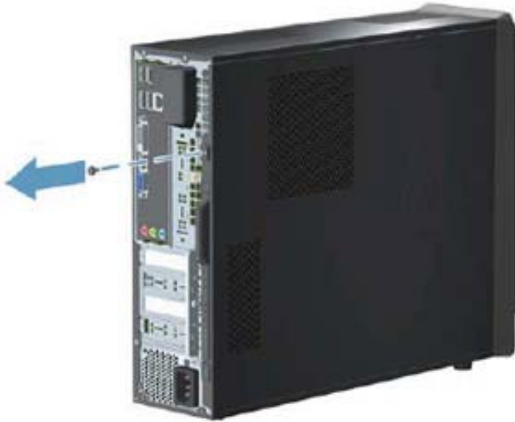
Figure 8-1 Removing the access panel screw
