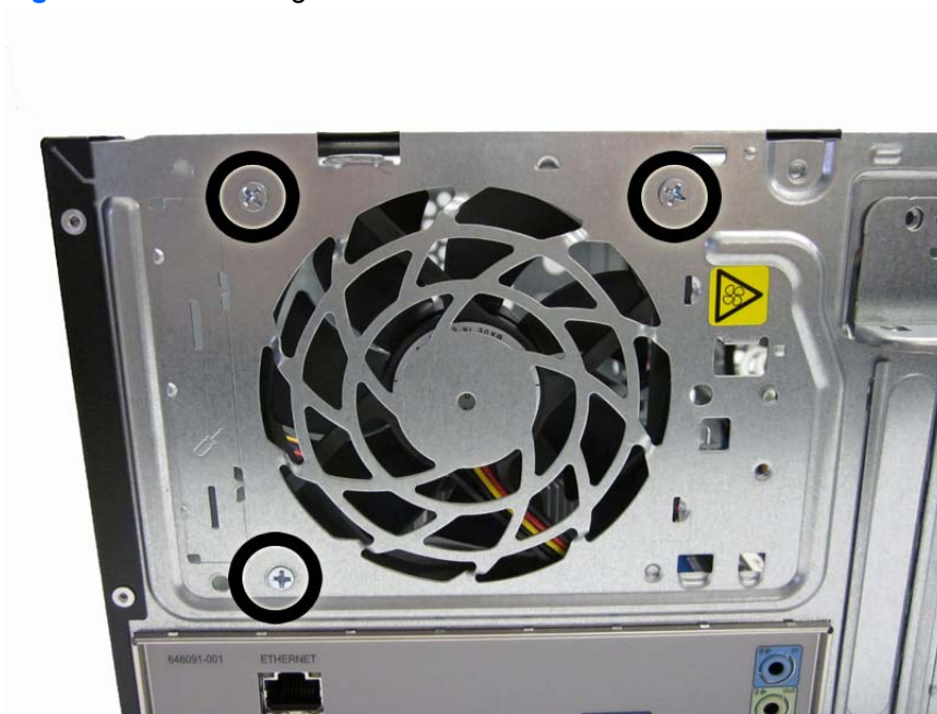
Figure 7-23 Removing the fan
