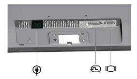
3. Connect one end of the analog signal cable to the monitor D-SUB connector and the other end to the computer.
