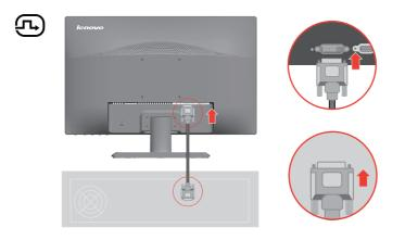
5. Insert the power cord into the monitor, then plug the monitor power cord and the computer cord into grounded electrical outlets.
