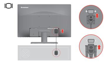
4. Connect the digital cable to the DVI connector of the monitor and the other end on the back of the computer.
