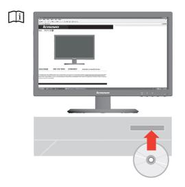
8. To optimize your monitor image, press the Automatic Image Setup key. Automatic image setup requires that the monitor is warmed up for at least 15 minutes. This is not required for normal operation.
