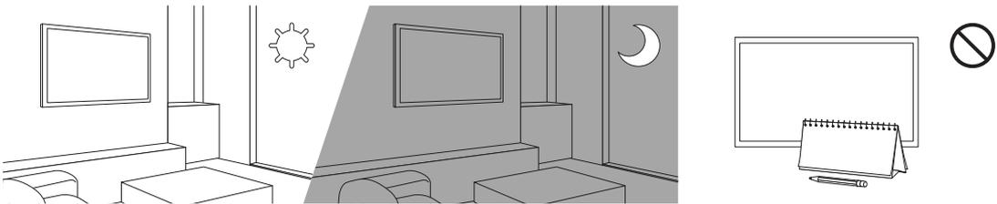
Eco Sensor adjusts the brightness of the TV automatically. This feature measures the light in your room and optimizes the brightness of the TV automatically to reduce power consumption. If you want to turn this off, go to (🏠) > ⚙️ Settings > General > Eco Solution > Ambient Light Detection.
