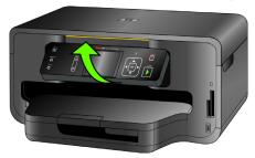
To adjust the control panel position:
