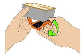
7 Insert the ink cartridge into the printhead.
