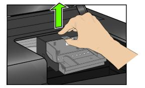
**5** Remove the old printhead from the carriage.
