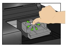
10 Reinstall the ink cartridges. As needed, see "Replacing ink cartridges" on page 62.
