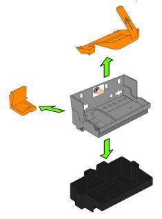
8 Place the new printhead into the carriage.
