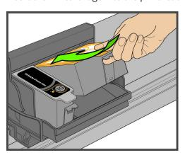
8 Press down on the tab until you hear a click and feel the latch snap into position.
