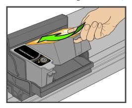
Listen carefully during this step; make sure you hear the ink cartridges click into place in the printhead. This seats the cartridges properly, and prevents ink from being dispensed incompletely on your print or copy jobs.
