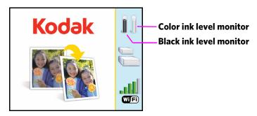
The first time you use your Kodak ESP 7 All-in-One printer and press the **Menu** button (described on page 11) on the control panel, the Main menu displays on the LCD screen.
