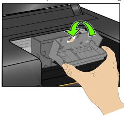
9 Push firmly against the target label on the printhead until you hear it click into place.
