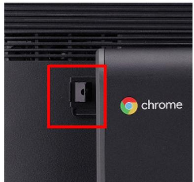
6. Tighten the VESA lock bracket and VESA bracket with provided hexagon screws or phillips screws depending on package contents.
