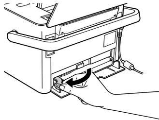
Caution: Do not try to pull out the cartridge without moving the lever.
