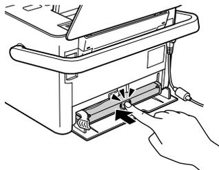
Note: The cartridge won't go in all the way. You need to use the cartridge lever to lock it in place.
