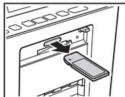
**Bottom slot:** Push in and release the card release button so it pops out. Then push in the button again to eject your card and pull it straight out of the slot.
