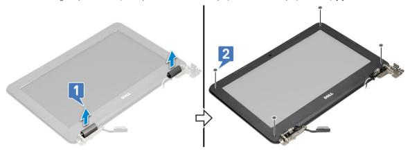
Remove the four M2.5x3.5 screws and pry the edges to release the display bezel from the display assembly [2,3].
