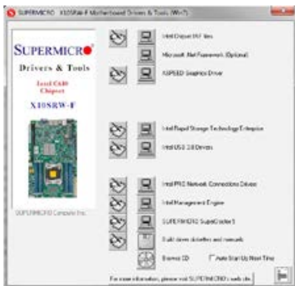
Figure 5-7. Driver/Tool Installation Display Screen
