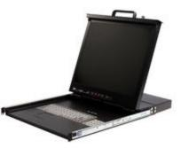
The RACKCONS1908 1U 19-inch Rack Mount LCD Console provides centralized control for servers and KVM switches with an integrated 8-port KVM switch, a 19-inch LCD monitor, full 106-key keyboard and touchpad, neatly combined into 1U of rack space for any standard rack or cabinet 30-inches (or greater) in depth.
