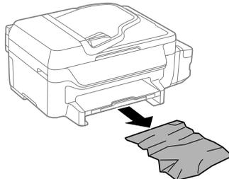
Remove the auto-duplexer from the back of the printer and remove any jammed paper.
