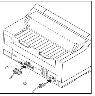
Make sure that the printer is set to the correct voltage (e.g. 230 V in Europe, 120 V in the U.S.A.). To do this, check the plate above the power inlet at the rear of the printer.
