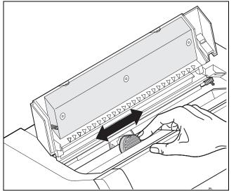
Move the print head carriage back and forth several times. If the ribbon is correctly seated, there must be no perceptible resistance.
