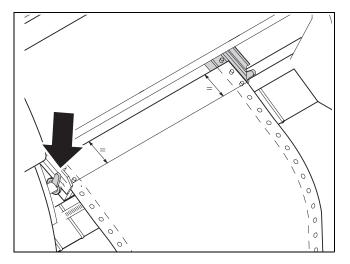
Open the coloured latch lever and align the tractor so that the first printing position on the paper matches the **X** mark on the printer housing.
