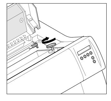
Insert the coloured tension knob into one of the two locations.
