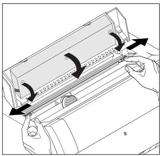
Press the friction mechanism down until it clicks into place.
