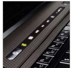
8-button EasyControl Bar including Eco Utility Button
