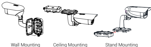
Figure 2-21 Installing Junction Box Cover
