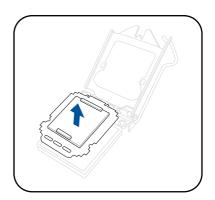
Position the CPU above the socket, ensuring that the gold triangle mark is on the bottom-left corner of the socket, then fit the CPU notches to the socket's alignment keys.
