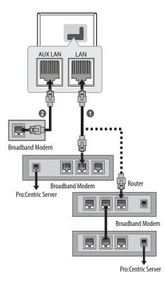
Connect the LAN port of the Modem or Router to the LAN port on the TV.
