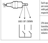
Each up/down pins are connected to CPU with pull up resistor respectively.
