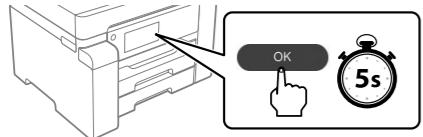
When the message of seeing **Start Here** is displayed, press **OK** for **5 seconds**.
