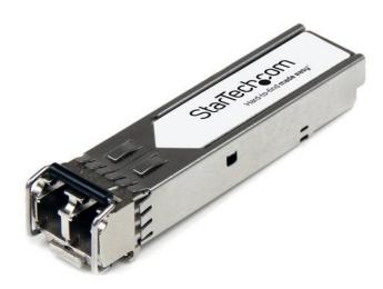
The 10G-SFPP-SR-ST is a Brocade 10G-SFPP-SR compatible fiber transceiver module that has been designed, programmed and tested to work with Brocade brand switches and routers. It delivers dependable 10 GbE connectivity over fiber cable, for 10GBase-SR compliant networks, with a maximum distance of up to 200 m (656 ft).
