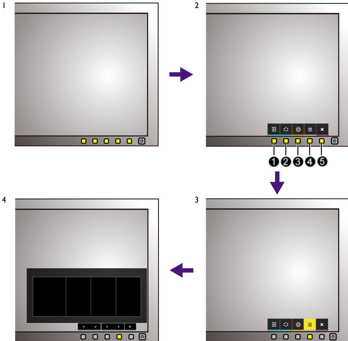
1. Press any of the control keys. Alternatively, press the **OK** key on the Hotkey Puck.
