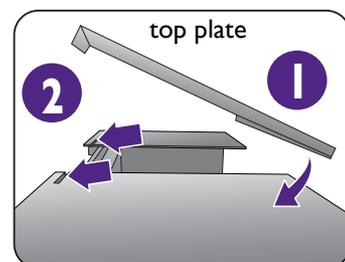
7. If you intend to calibrate the display's color by a colorimeter, slide to open the cover on the top plate so the colorimeter can be installed.
