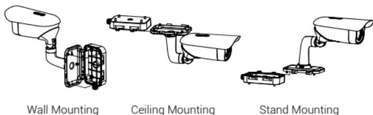
Figure 2-10 Installing Junction Box Cover
