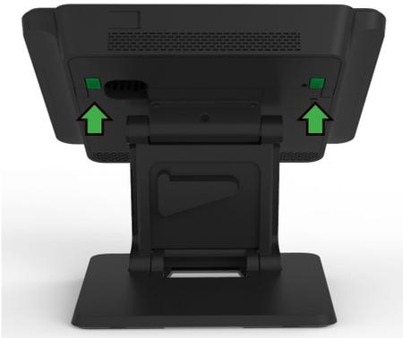
Tilt the display back to access the I/O connections and remove the cable cover.
