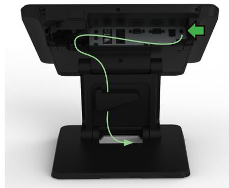
Connect the power cable to the DC power jack marked by the arrow. Then route the cable through the cable clips and through the bottom of the stand.
