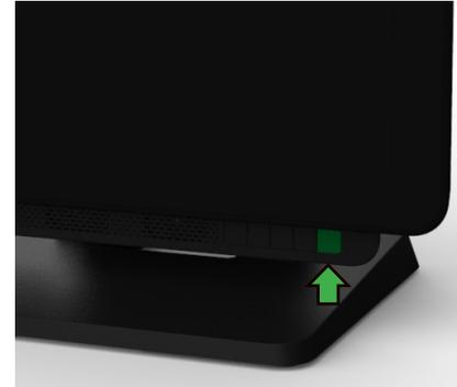
The power button is located at the bottom as shown.
