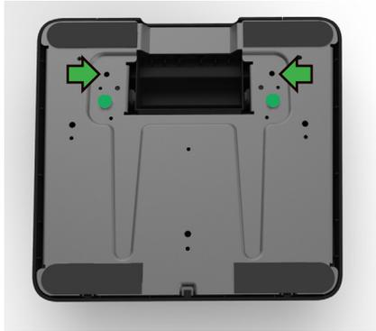
The stand supports both upright and lowered orientations. The stand is set to the lowered position from the factory. Change the orientation to upright by removing the green colored screws from the bottom of the stand and install them in the location marked by the arrows
