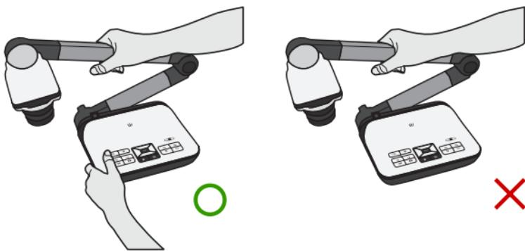
3. The camera can be damaged if it hits a desk surface or any hard object.
