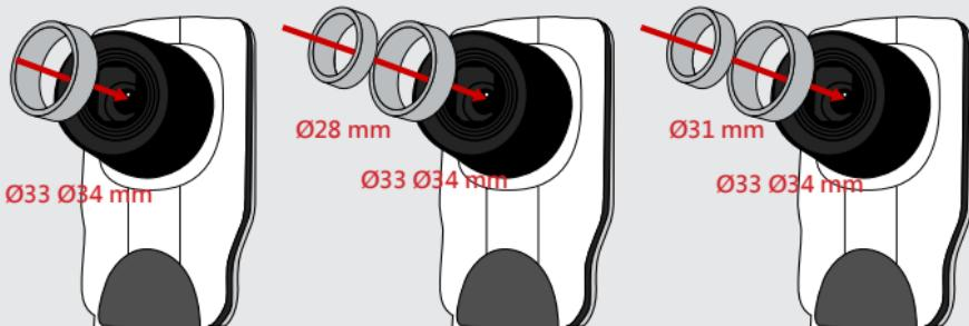
4. Mount the microscope adapter onto the Lens.
