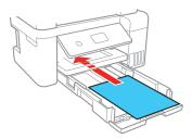
**Note:** Make sure the paper is loaded against the front edge guide and not sticking out from the end of the cassette.
