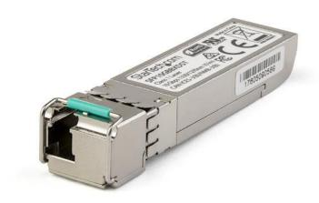
The SFP10GBX40DS is a Dell EMC SFP-10G-BX40-D compatible downstream fiber SFP transceiver which pairs with StarTech.com's SFP10GBX40US. They are designed, programmed and tested to work with 10GBase-BX40 compatible Dell EMC switches and routers. The SFP+ transceiver module supports a maximum distance of up to 40 km (24.8 mi) and delivers dependable 10 GbE connectivity over fiber cabling.
