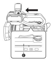
5 While pressing the handle unit mounting screw down, turn it in the direction indicated by arrow 2 until it stops.
