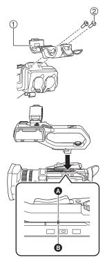
f 4 Slide the handle unit in the direction indicated by the arrow.
