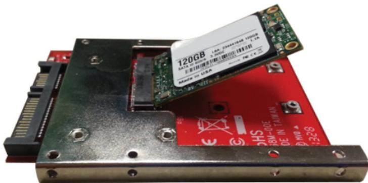
2. Press the drive down toward the drive mounting bracket, and drive the two smaller screws included in the screw kit through the mounting holes on your SSD drive and into the drive mounting bracket using a Philips head screw driver (not included).
