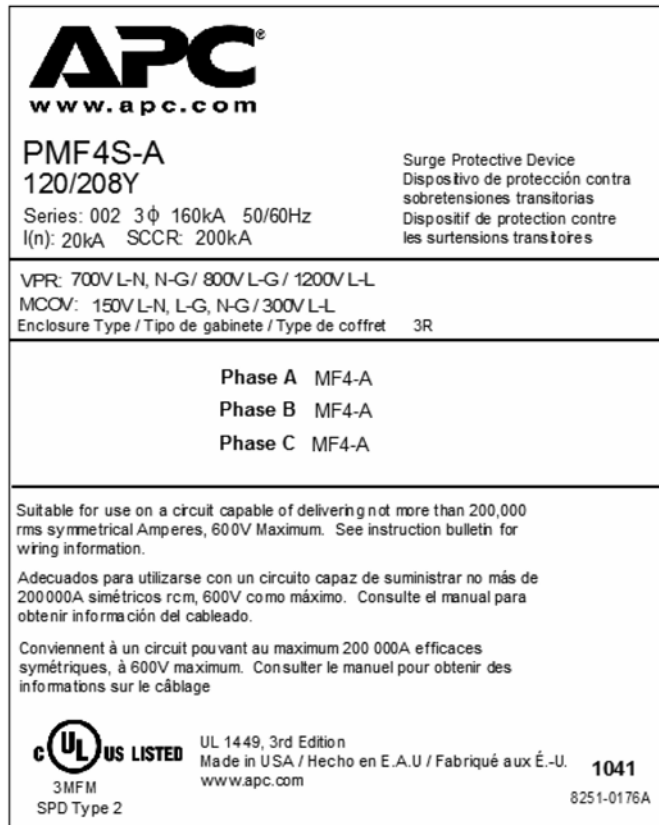
Figure 1: SPD Nameplate Example
