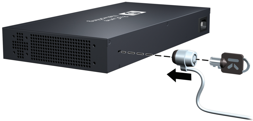
Figure 2-11. Using a Security Cable with the 1410-24G Switch
