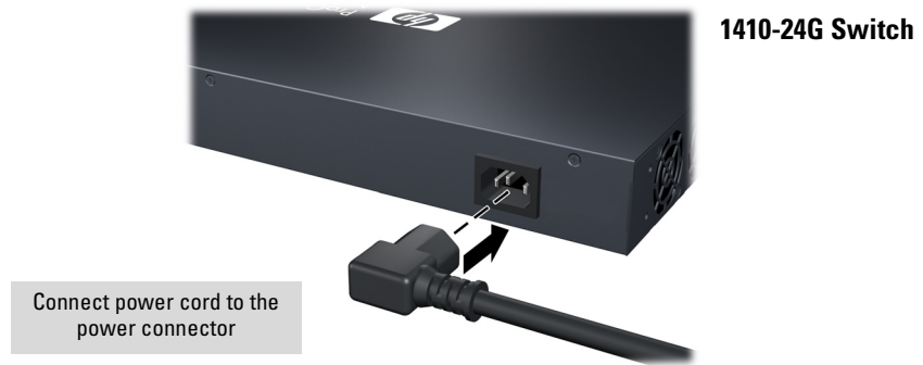
Figure 2-2. Connecting the 1410-24G Switch power cord
