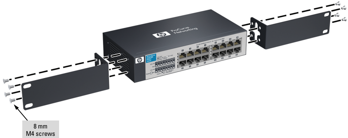
Figure 2-4. Attaching mounting brackets to the 1410-16G Switch
