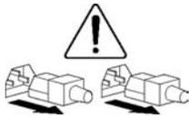
These symbols, on power supplies or systems, indicate that the equipment is supplied by multiple sources of power.
