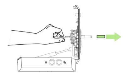
6. Rotate the Bat Top Joystick Grip onto the joystick shaft until it is securely fastened.
