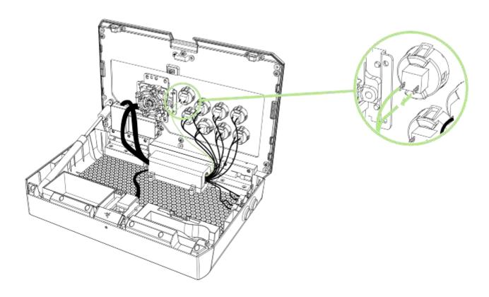
4. While holding the action button's fastener, push the action button out. You can use the screwdriver to push the fasteners in more easily if needed.
