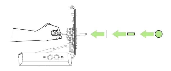
19. Reattach the cables to the action buttons.
