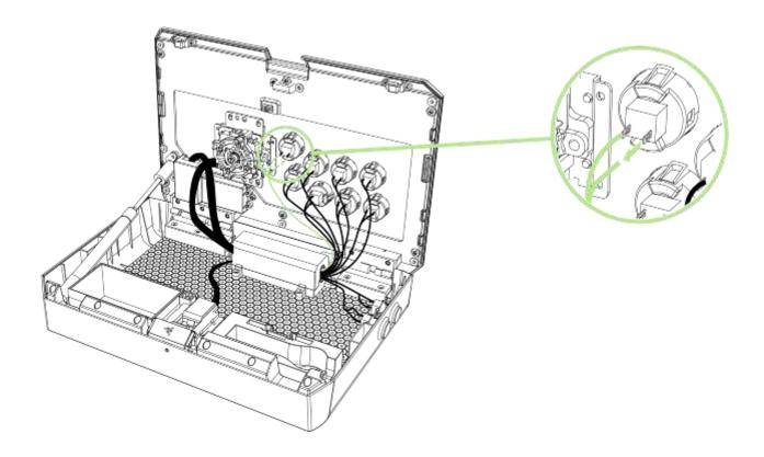
20. Ensure that all cables are properly connected then close the lid.
