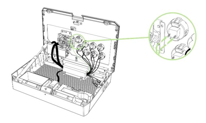
8. Ensure that all cables are properly connected then close the lid.
