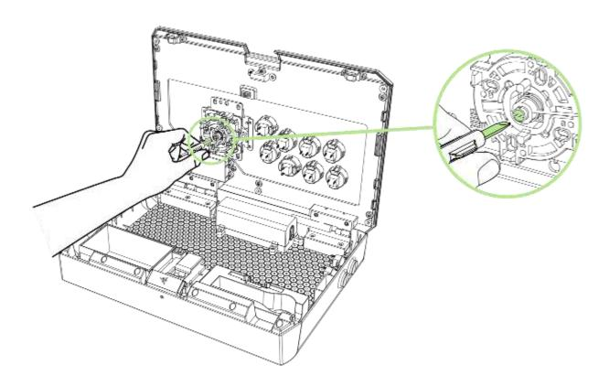
4. Rotate the Ball Top Joystick Grip until it is removed from the joystick shaft.
