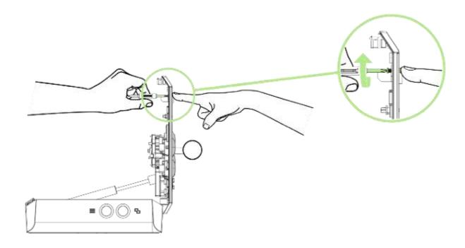
10. Repeat step 9 until all six screws and metal stoppers are removed.
