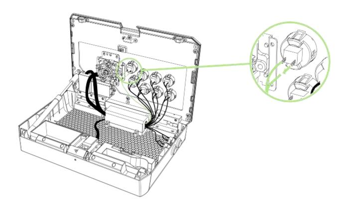
7. While holding the action button's fastener, push the action button out. You can use the screwdriver to push the fasteners in more easily if needed.
