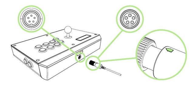
6. Rotate the tip clockwise until the detachable cable is firmly connected to the Razer Atrox for Xbox One.
