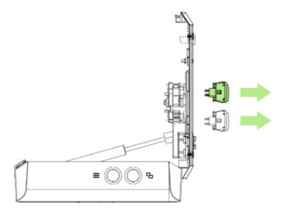
6. Insert your desired action buttons or button covers\* into the slots.
