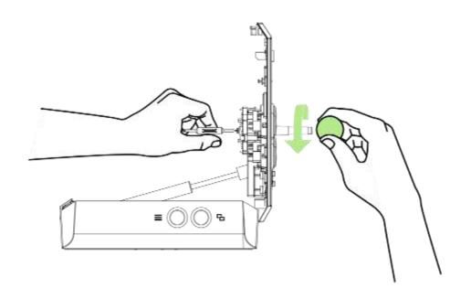
5. Remove the shaft cover and dust washer from the joystick shaft.
