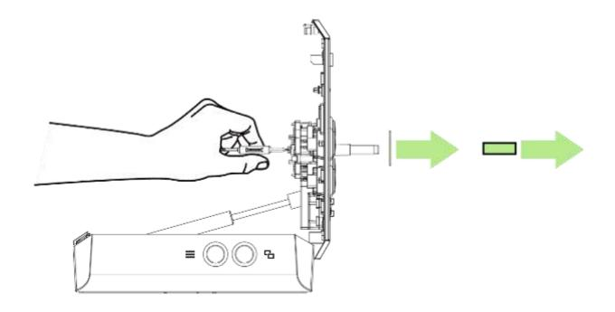
6. Carefully remove the cables from the action button.
