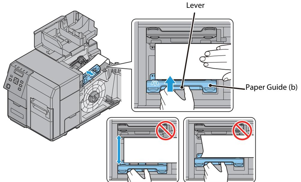
11. Insert the end of the paper into the paper feed slot. The paper starts to feed automatically after a certain amount is inserted.
