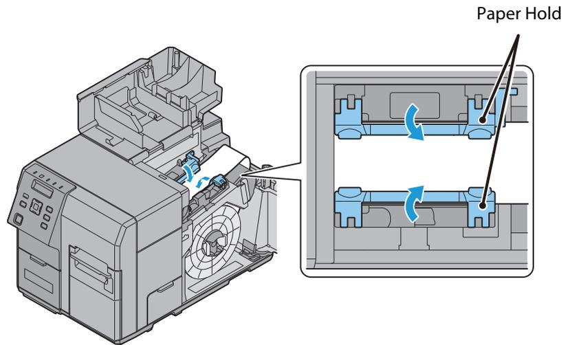
13. If the paper is loose, turn the roll paper flange in the direction of the arrow to tighten the paper.
