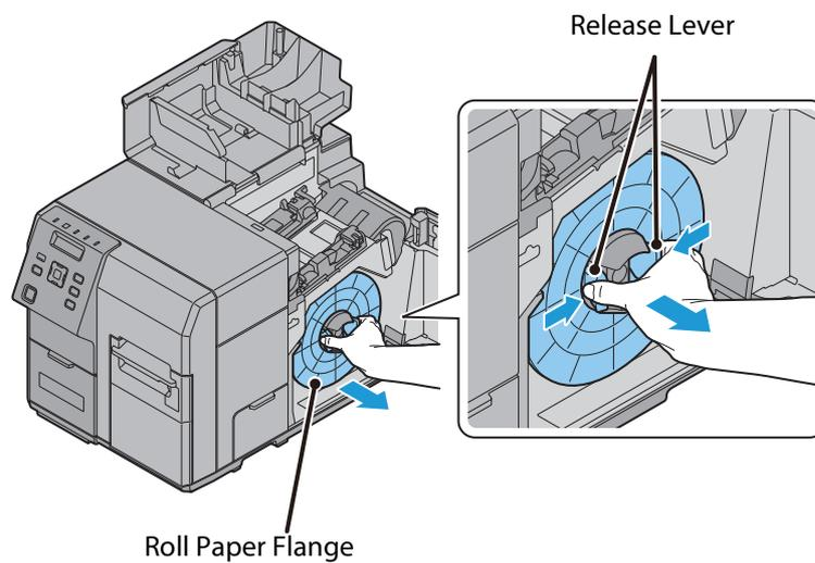
5. Attach the roll paper to the spindle, and push the core of the roll paper as far as possible so that it is securely fit it into place.
