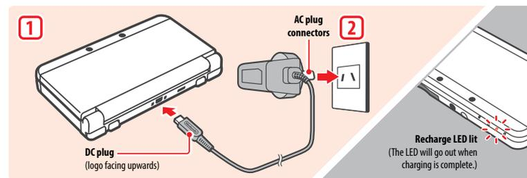
**1 Connect the DC connector plug to the system**
