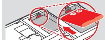
Note: Ensure that the battery is facing in the right direction.
