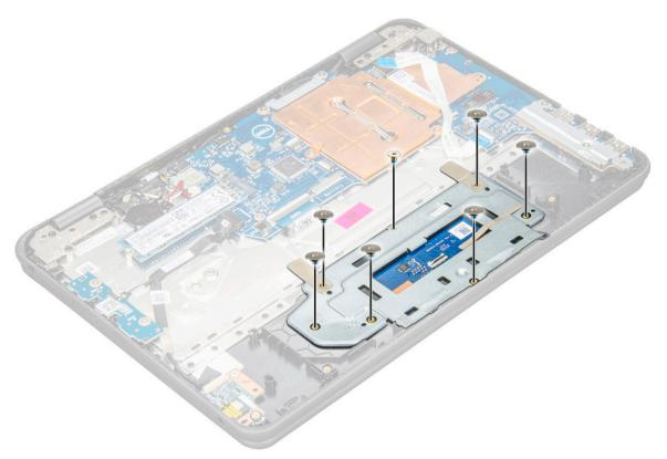
b Remove the adhesive tapes securing the bracket to the touchpad [1]. Lift the bracket away from the system [3]
