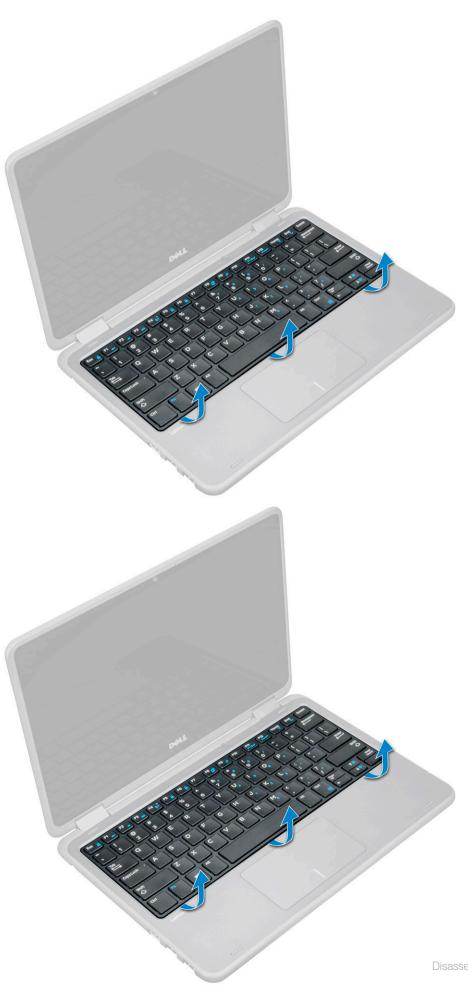
6 Slide the keyboard outwards, away from the computer, and lift the keyboard away from the computer.
