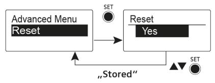
When you reset the plug-on transmitter, only the selected settings of the pilot tone and the  ${\bf U}$  frequency bank are retained.
