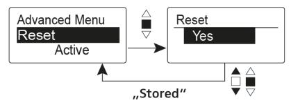
When you reset the wireless microphone, only the selected settings of the pilot tone and the  ${\bf U1}$  to  ${\bf U6}$  frequency banks are retained.
