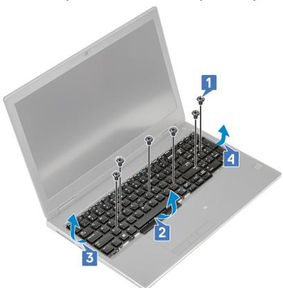
g Slide and remove the keyboard from the system.
