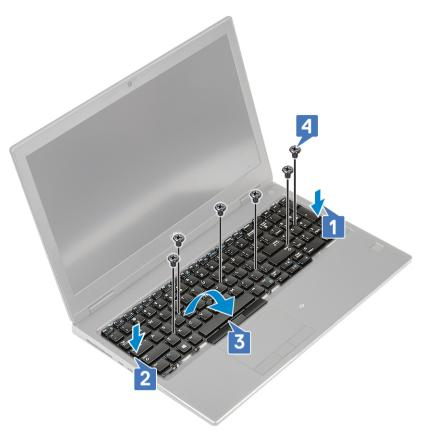
d Align the keyboard lattice to its position on the keyboard and ensure that the keyboard lattice clicks into its place.
