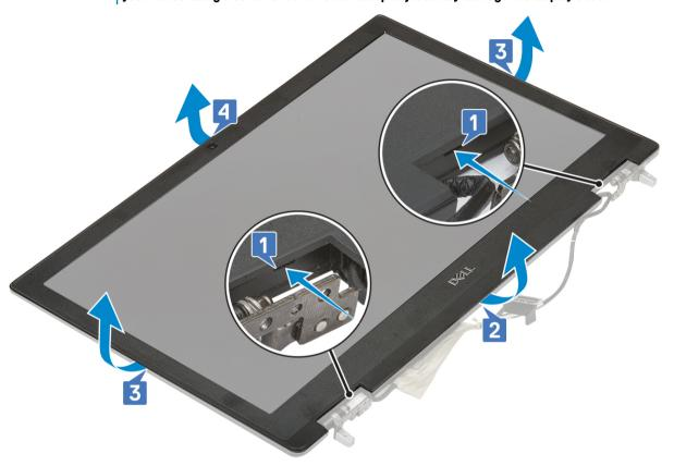
NOTE: The display bezel shipped with a non-touch display is a disposable part and should be replaced with a new display bezel anytime it is removed from the system.
