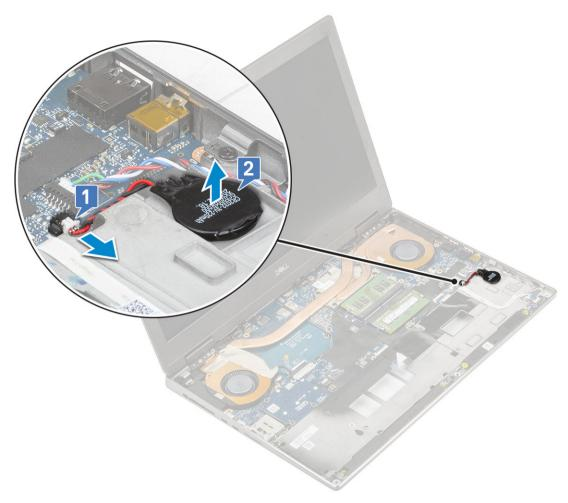
CAUTION: Disconnecting coin cell battery may reset BIOS settings, time and date within System Settings, cause BitLocker or other security resets.
