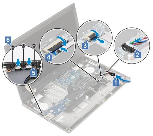
f Connect the power connector cable to the connector on the system board.
