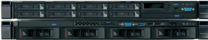
The versatile 1U, two-socket Lenovo System x3550 M5 rack server fuels almost any workload from infrastructure to Big Data with leading security, efficiency and reliability. Integrated with up to two Intel Xeon E5-2600 v3 series processors, faster, energy-efficient TruDDR4 Memory and up to 12 storage drives, the x3550 M5 delivers exceptional performance.
