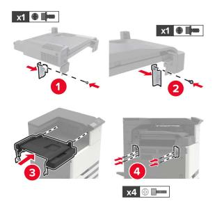
Attach the finisher to the printer.
