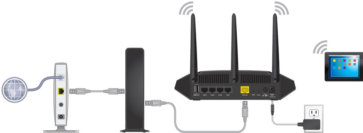
Figure 4. Connect the access point/router to another router in your network
