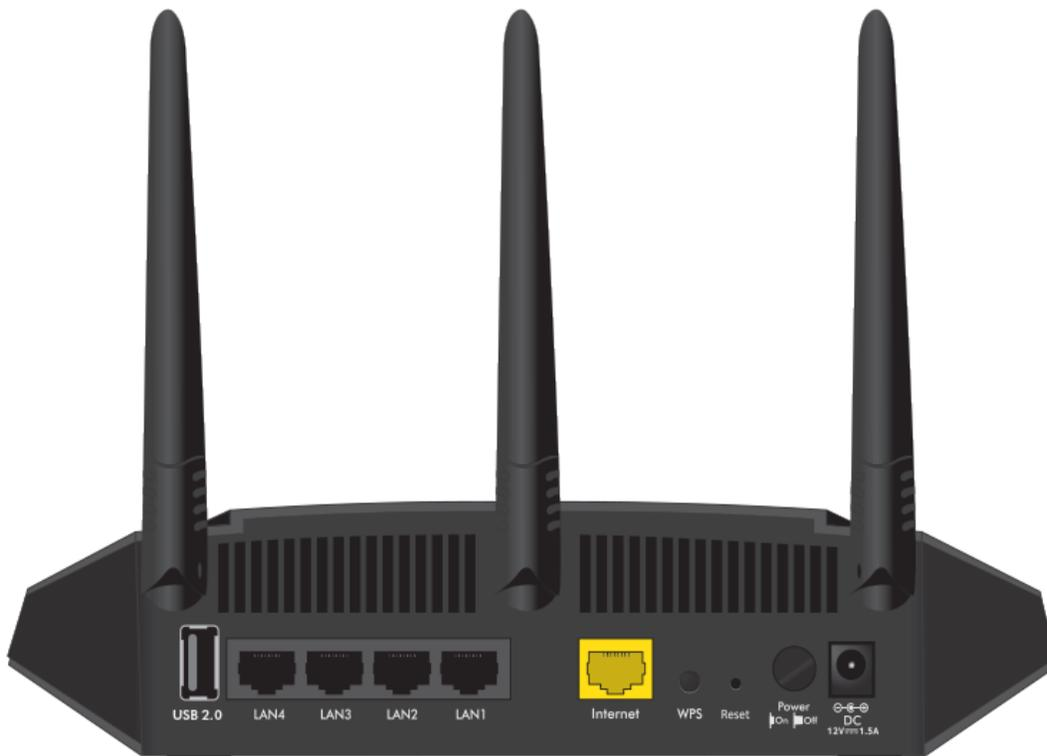
Figure 2. Access point/router back panel
