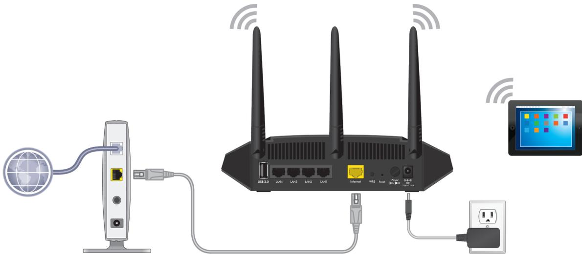
Figure 5. Connect the access point/router in router mode to your Internet modem
