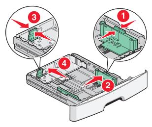
If you are loading a longer size of paper like A4 or legal, squeeze the length guide tab and slide the length guide backwards to the position for the length of paper you are loading. The tray extends backwards as shown.
