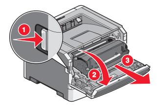
2 Lift the flap in front of the printer, and then remove any jammed sheets.
