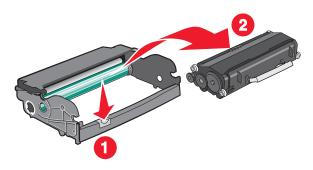
**4** Unpack the new photoconductor kit. Be careful not to touch the photoconductor drum.
