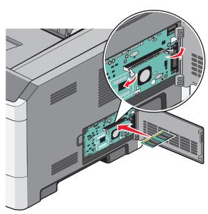
**4** Push the memory card into the connector until the latches *snap* into place.
