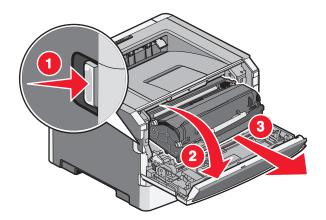
4 Lift the flap in front of the printer, and remove any jammed sheets.
