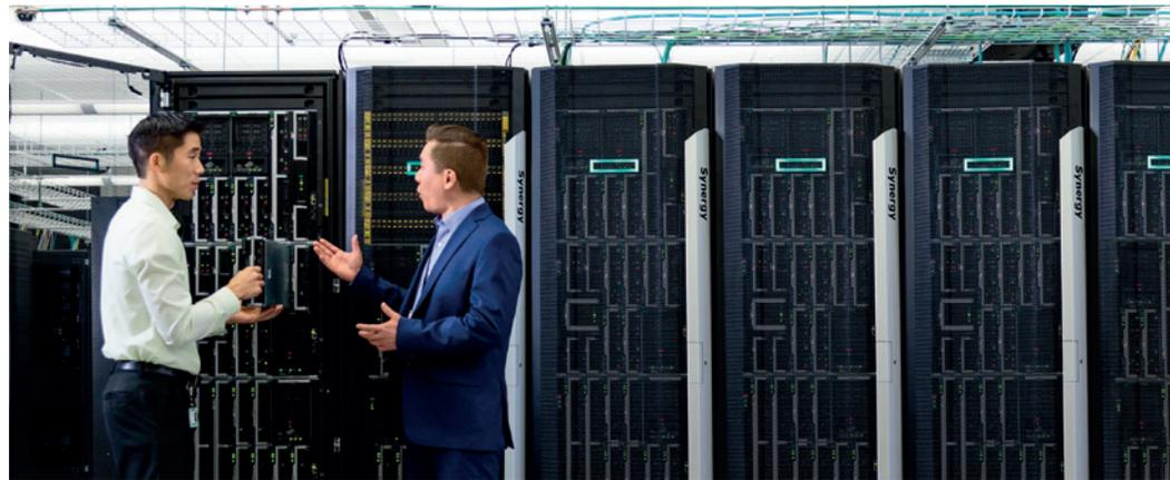
JR East Japan Information Systems Company (JEIS) has fully adopted open source software to develop a business-critical fault information system on the HPE Moonshot System ultra high-density server platform. The company consolidated all the functions required for the fault information system into a single 4.3U Moonshot 1500 Chassis populated with 45 HPE ProLiant m300 Server Cartridges.
