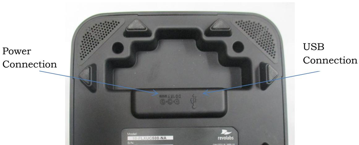
**Figure 2: FLX UC 500, Connector View**
