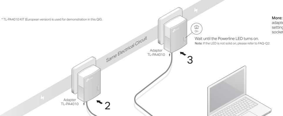
More: To add additional Powerline adapters and extenders with the default settings, simply plug them into the wall sockets on the same electrical circuit.
