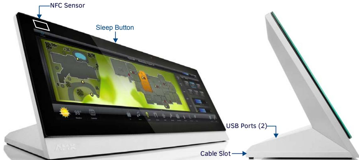
FIG. 8 MXT-1900L-PAN - Front View
