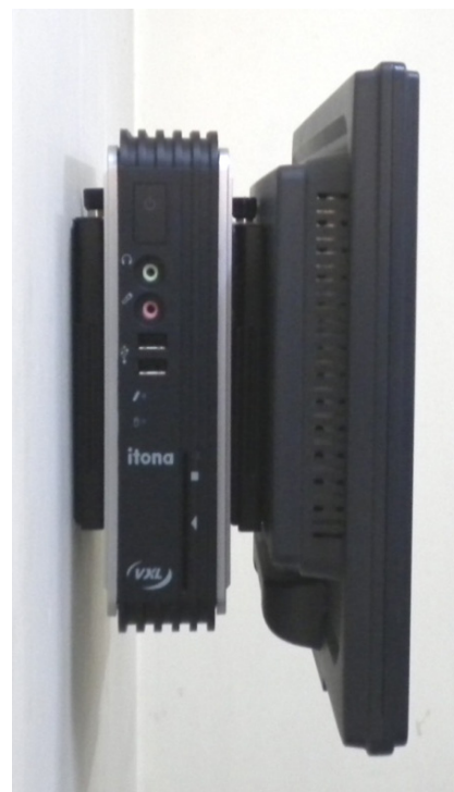
Figure 2-10: Wall Mounted Client and Monitor
