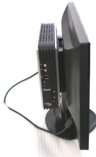
Figure 2-8: Mounting the Thin Client using a VESA
