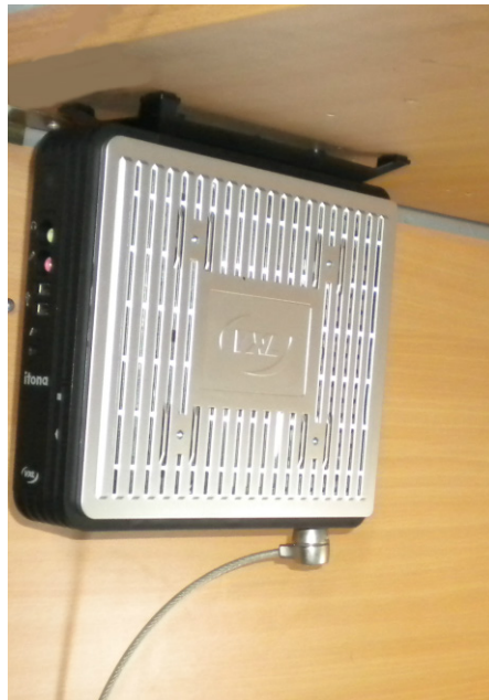
Figure 2-18: Kensington Lock Slot on the Bottom Strip
