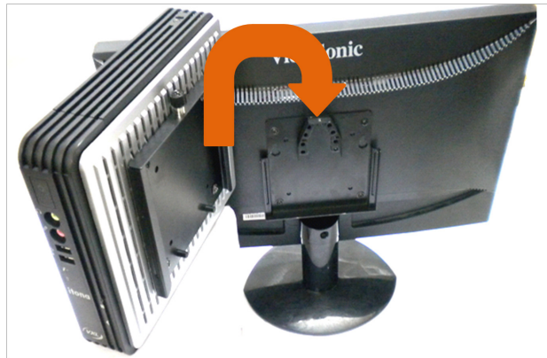
Figure 2-8: Mounting the Thin Client using a VESA
