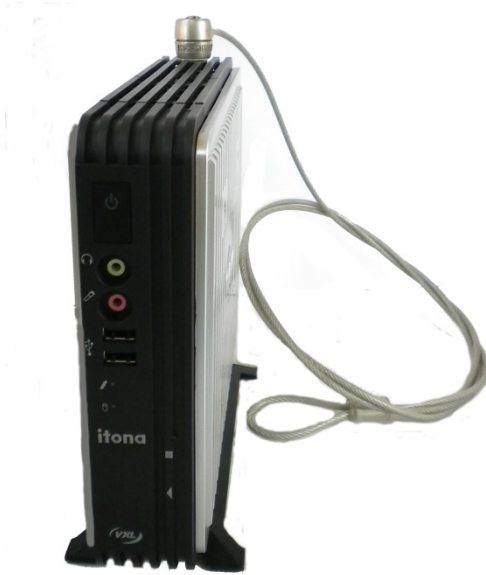
Figure 2-17: Kensington Lock Slot on the Top Strip
