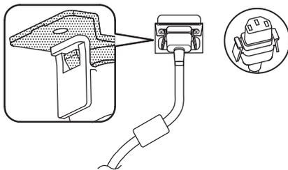
3. To unplug the AC cord, press the two knobs and pull.
