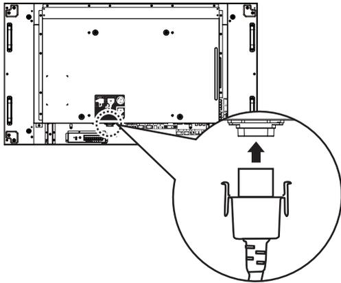
2. Plug the AC cord firmly until it clicks into position. Make sure the AC cord is locked on both the left and right sides.
