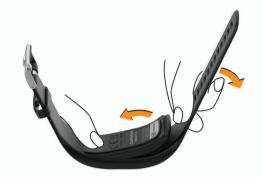
**2** Insert the device into the band, and stretch the band material around the device.
