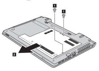
**5** Remove the screw shown in the illustration **3**.
