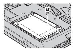
Remove the hard disk drive by gently pulling in the direction of the arrow.
